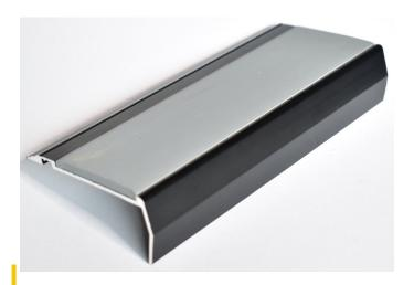
At ATB, our wide range of aluminium stair nosing ensures a suitable product is available for whatever the situation whether vinyl, concrete, carpet tiles or timber. The aluminium base can be screw fixed and the PVC infill ensures the fixings are hidden.
